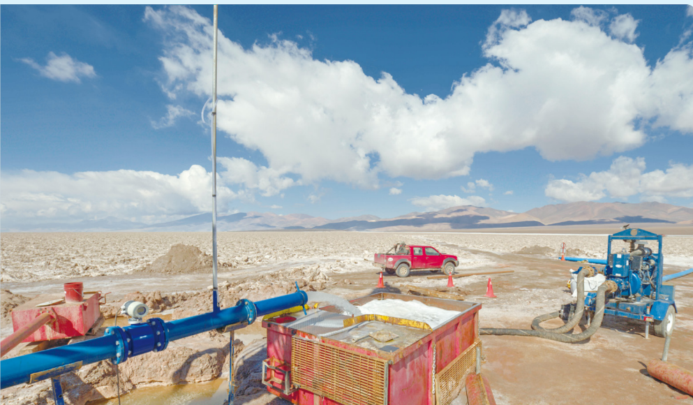
Extraction of lithium components from the groundwater beneath the massive salt flat
