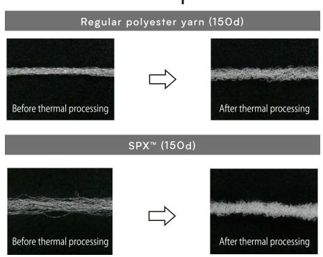
Develops a spring-like crimp and puffiness when heated
